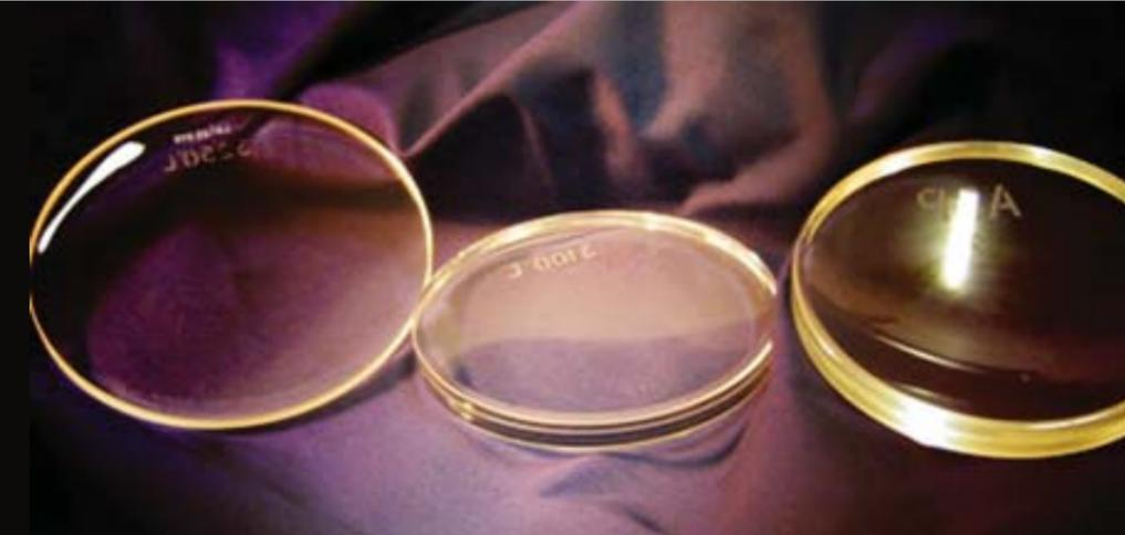
Crossbows Optical has been manufacturing ophthalmic glass moulds since the 1980s and developed their own state of the art design technology using precision glass grinding and polishing machines. Progressive, aspheric and atoric moulds are sold worldwide for semi-finished and finished lens production.
